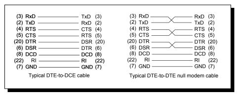
Figure 13 --- Cabling requirements for RS-232-C devices (cables using 25-pin connectors shown)
